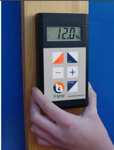
A hand holds the FMW-B moisture meter against a wooden surface. The LCD screen displays 12.0%.     |
