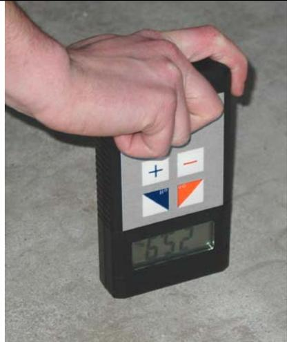
A hand holds the FMW-T moisture meter against a concrete surface. The LCD screen displays 65.2%. |
